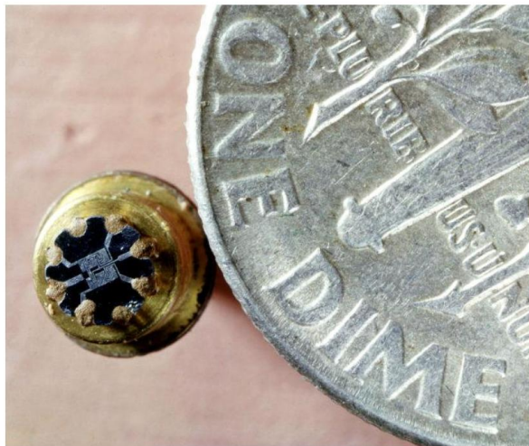
Fairchild's first IC, the “F” element flip-flop compared to a dime coin. Photo: Getty Images
